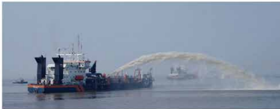
Process: Sand is sprayed in a strategic spot in the sea to a mountain / The sea moved the sand to where it is needed
