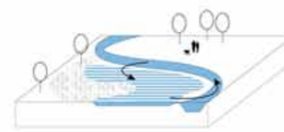
Transformation strategy : floodplain restoration Model 1, transformed the green area (nature, park, sports field) into a water park by excavating land and expanding the riverbank planted with reed systems.
